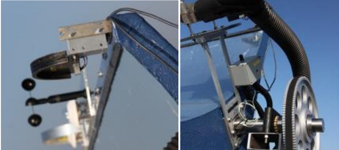
Figure 21: Sensory based tracking unit with two small PV units and the control box [14].
