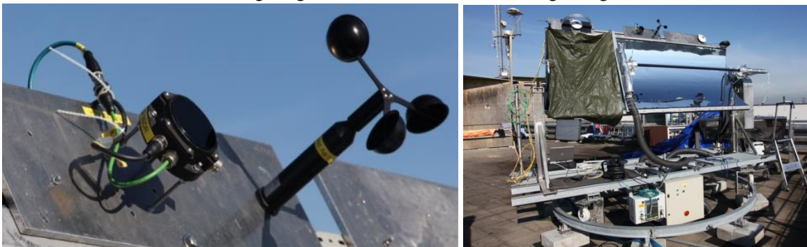
Figure 22: Installed Heliosensor in the aperture area of a collector (detail (left) and general view (right)) [14].
