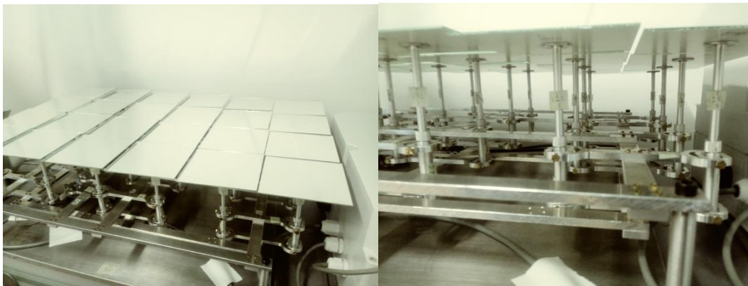
Figure 4: View of a prototype mirror module with nearly parallel mirrors
